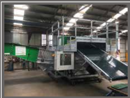
TCI’s D8 Decorticator, an example of the type of machine needed to process hemp stalks into fibre and hurd.
