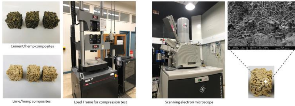
Compressive strength test
