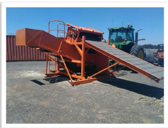
D8 installed for use powered by the PTO of a tractor. Developed by TCI.
