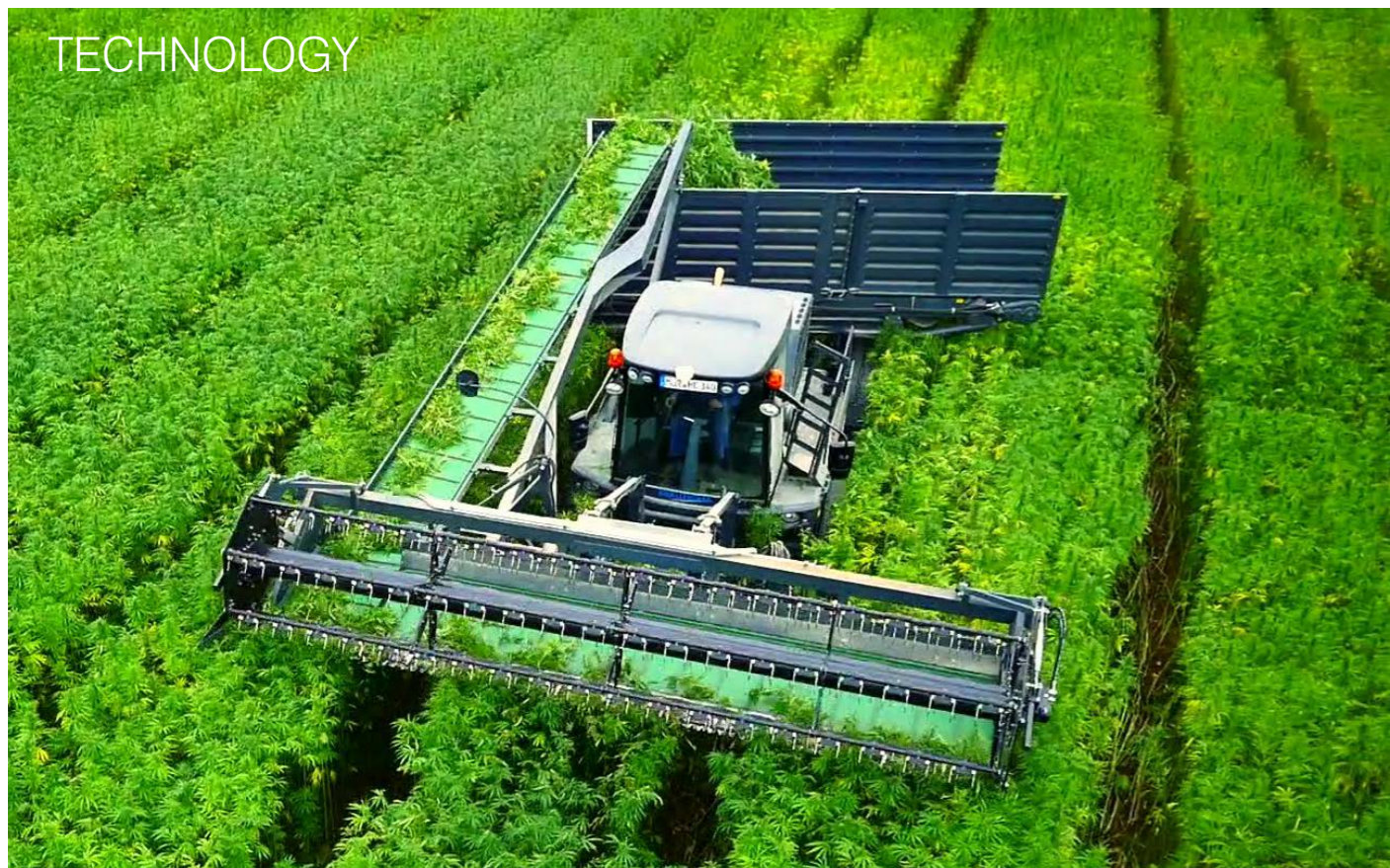
The MC HC 3400, which undergoes constant refinement, has been successfully deployed in hemp fields the last 5 harvest seasons.
